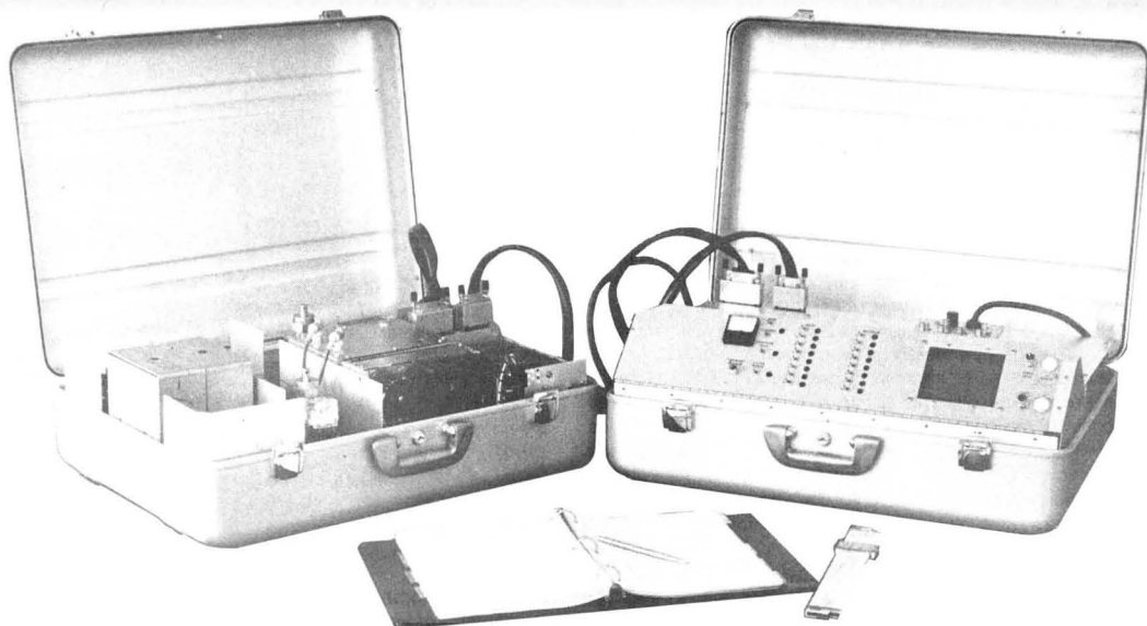
Figure 1. Suitcase (right) shows the operator's control panel and CRT monitor; suitcase (left) with protective insulation and covers removed shows the quadrupole analyzer and its vacu-
